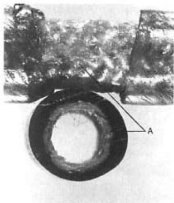
Figure 2. Cutaway (upper) and cross-sectional (lower) views of an Eschmann tracheal tube introducer. A = braided Dacron core.
